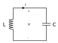
Because we have connected the inductor and capacitor together, we must equate the two reactances,  $X_L$  and  $X_C$ .
