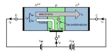
Looking at the way the currents flow through the device, we can say the emitter current  $(i_E)$  is equal to the sum of the base current  $(i_B)$  and collector current  $(i_C)$ .
