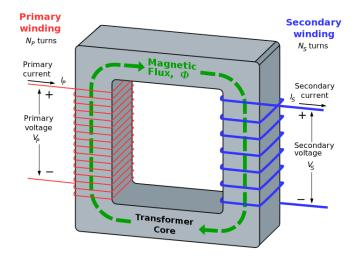
The voltage and currents in the primary and secondary windings are scaled by the ratio of turns on the primary winding  $(N_P)$  and the secondary winding  $(N_S)$ . Firstly the voltages:
