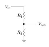
The derivation is out of the scope of this guide, but is explained in the book. The derivation is unimportant for the Full Radio Amateur's exam, as you are given the following formula on the formula sheet. What matters is that given two values for  $R_1$  and  $R_2$  you and  $V_{in}$ , you can calculate  $V_{out}$ .
