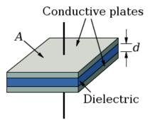
Using the formula below, you can work out the capacitance for a given place size of area A separated by a dielectric of parameter K and distance d.
