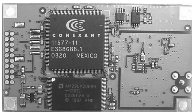
Figure 2. Jupiter GPS Receiver (Bottom View, Shown Approximately Actual Size)
