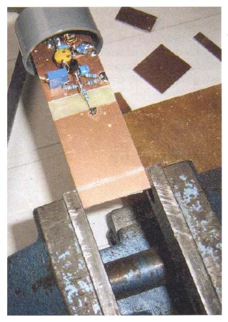
Photo 2 - Prototype of the pa0rdt-Mini-Whip ©.
