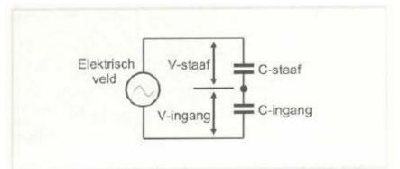
Figure 7 - Model of an active whip antenna.
