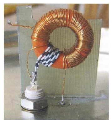
Photo 7 - 150:1 RF transformer for the passive antenna.
