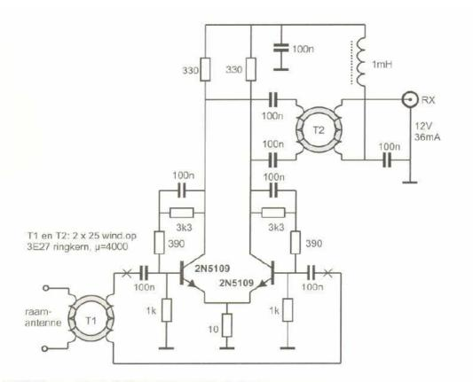
Figure 1 - Balanced active loop antenna.
