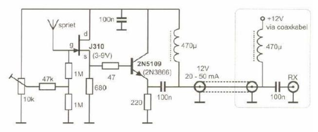
Figure 3 - Experimental version of the Mini-Whip.
