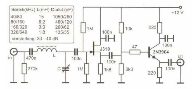
Figure 5 - Tunable preamplifier.
