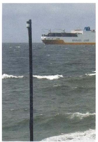
Photo 8 - Westkapelle, the Mini-Whip on a plastic mast section.
