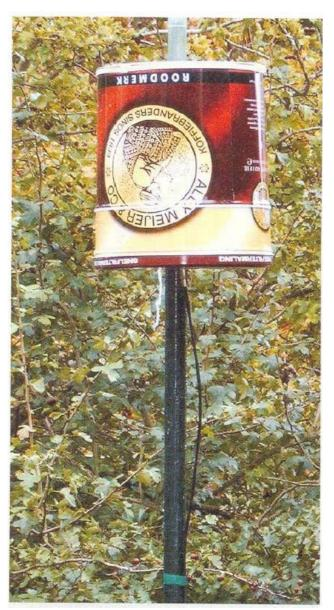
Photo 6 - Passive E-field antenna.
