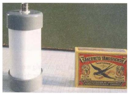
*Photo 3 - Standard form of pa0rdt-Mini-Whip* ©.
