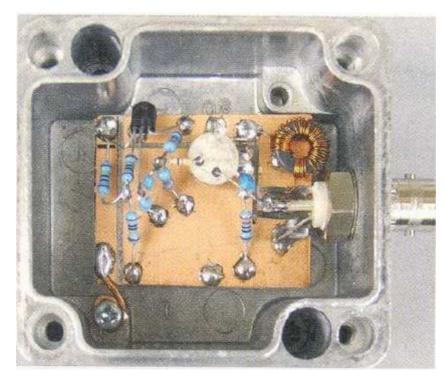
Photo 5 - Diecast-box Mini-Whip.
