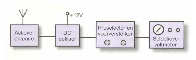
Figure 4 - The measurement setup.
