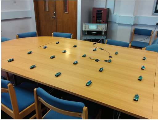
Figure 1: Example of our experimental setup. The 4 nodes located right-most in the image are used for monitoring purposes, with the RF signal generator used to generate interference shown in the background.
